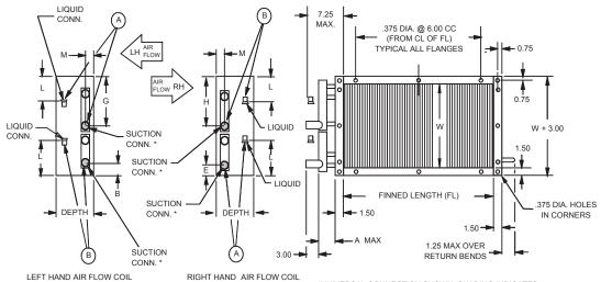
\*UNIVERSAL CONNECTION SHOWN. SHADING INDICATES CONNECTION FURNISHED WITH EACH UNIQUE COIL HAND.
