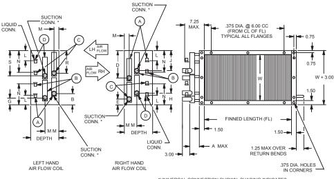
\*UNIVERSAL CONNECTION SHOWN. SHADING INDICATES CONNECTION FURNISHED WITH EACH UNIQUE COIL HAND.
