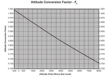
The CFM of standard air should be used to determine face velocity through the coil, which in turn is used to determine heat transfer values, and the air pressure drop through the coil.
