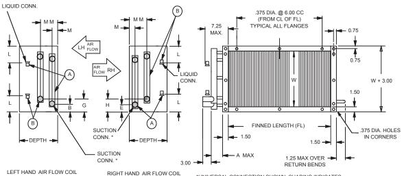
\*UNIVERSAL CONNECTION SHOWN. SHADING INDICATES CONNECTION FURNISHED WITH EACH UNIQUE COIL HAND
