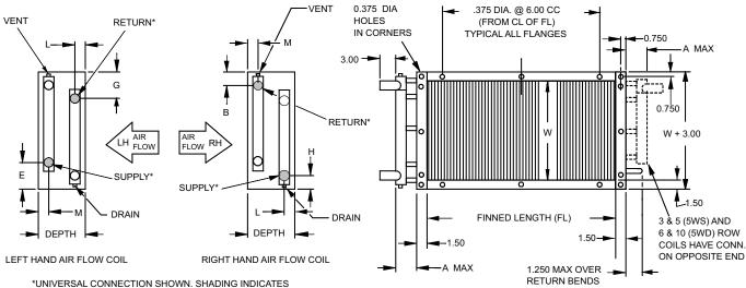
\*UNIVERSAL CONNECTION SHOWN. SHADING INDICATES CONNECTION FURNISHED WITH EACH UNIQUE COIL HAND.
